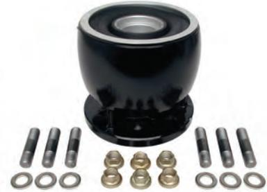
This coupler is used when a new replacement V6 or V8 Chevy with one piece rear main seal is used to replace an older V6 or V8 with a 2 piece rear main seal. (1986 & Up)
